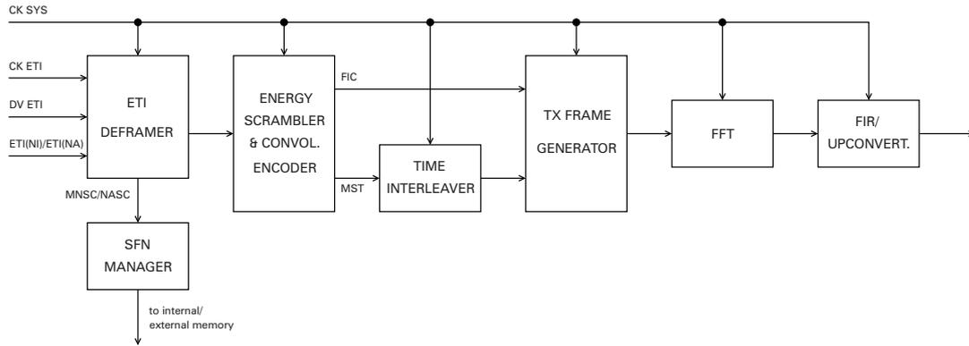
Figure 1: Block diagram of the DAB modulator
